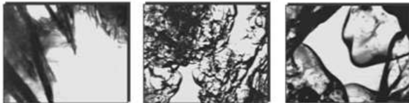
Figure 4 – Ice particles pictured through a microscope. (Left) Ice crystals formed from simply freezing water, they are rough and tend to clump. (Center) Ice particles formed from ice which has been shaved or crushed, rounder but still rough. (Right) Smoother ice crystals, as used in the slurry, formed by adding warm water to melt ice roughness or by adding a freezing point depressant. iii
